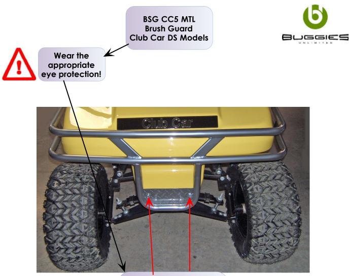
Remove the existing front Bumper. Set the new Brush Guard in place, bolt to the existing bumper mounting holes.
